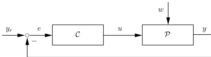
In the figure  $\mathcal{C}$  is an *error feedback controller*, which produces the input  $u$  of the system  $\mathcal{P}$  using the *regulation error*  $y - y_r$ . This kind of control structure is commonly used in practical applications such as in robotics and process engineering. Similar feedback structures can also be found in nature.
